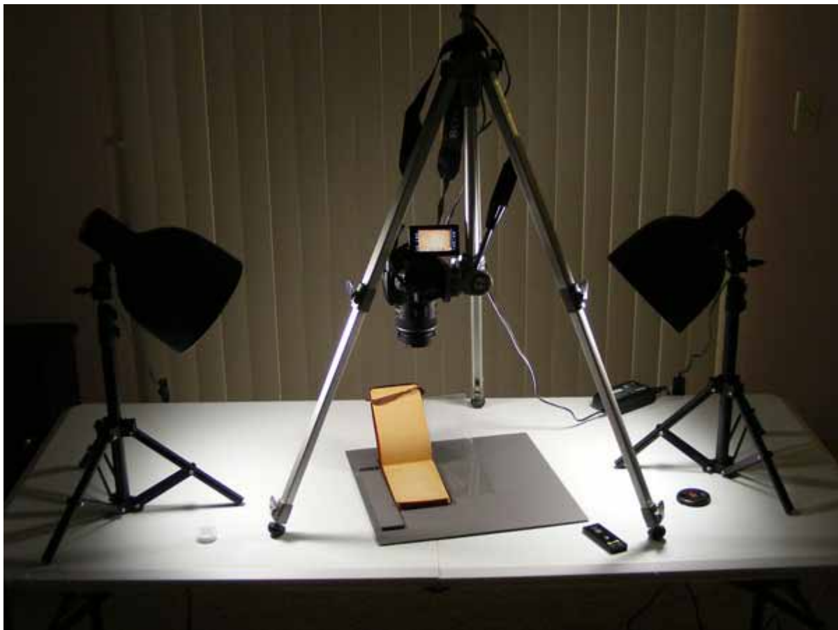
Figure D.1. An inexpensive copy stand using a camera tripod with photographic lights. The diary is supported by a piece of plastic to avoid being opened flat. The base is painted the color of a neutral gray card. The lights in the room are out to avoid contamination by extraneous light that does not match the temperature color of the photographic lights.
